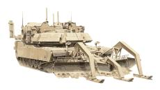
This heavily armored and highly mobile platform is equipped with a mine plow and demolition charge systems that would detonate Russian explosives from safe distances, clearing the way for follow-on combat formations to penetrate heavily mined areas of operation.
